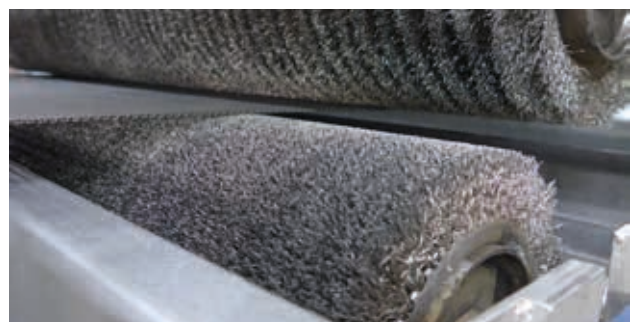
These pictures show essentials of a good brush system: upper & lower brush of different design
