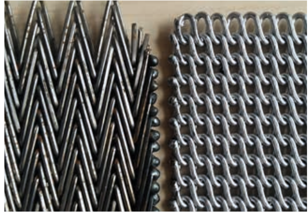
Balance weaved CB5 (left) replaced by Z-Belt F4018 (right)
