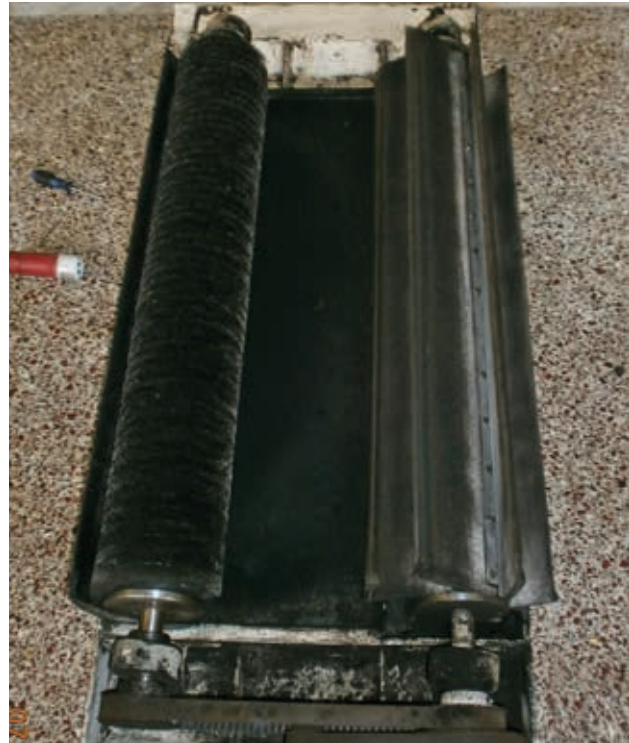
On the right a Flip-Flop needle felt cylinder can be seen (combined with a brush)
