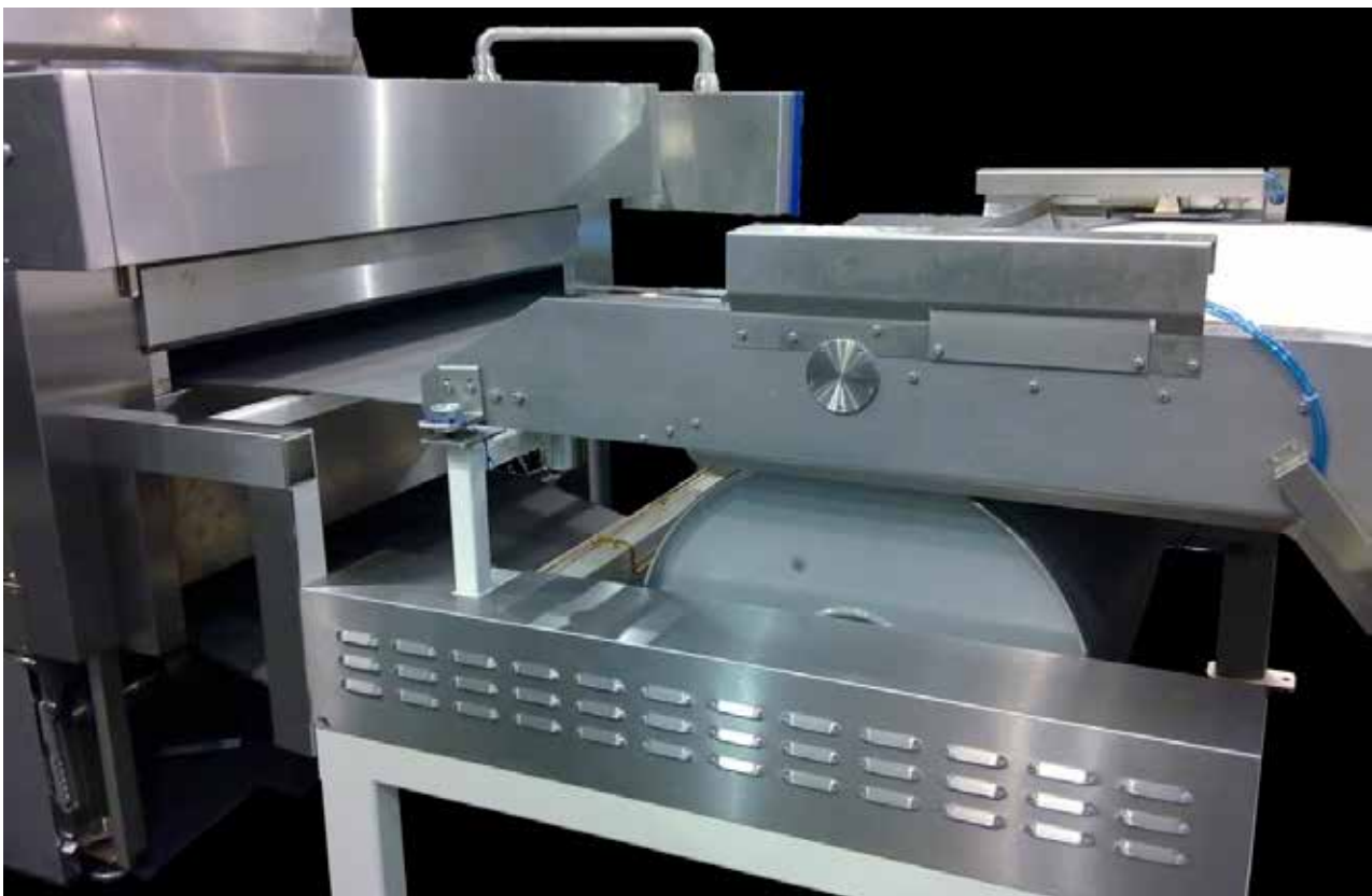
Oven feeding area with big diameter turning drum
