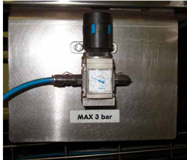
A good tensioning with an indicating label for the maximum force
