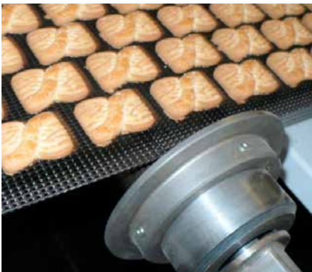
Example for guiding disc with a (good) distance to the belt edge
