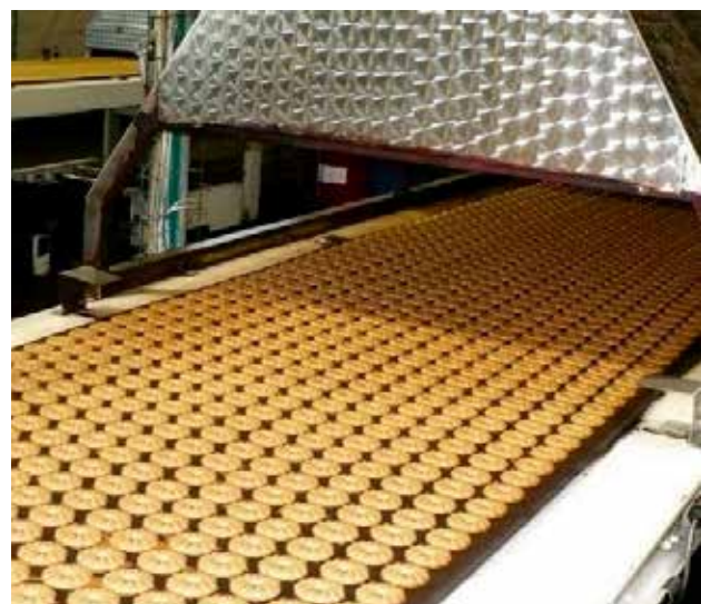
Example of a heat-covering roof at the oven's exit
