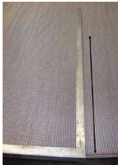
The same type of belt (with welded edges) showing a nearly perfect 90° row of meshes (and the angle metre to check it)
