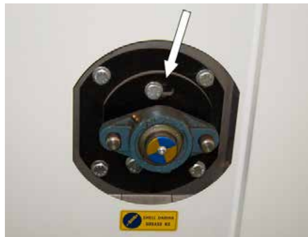
Support roller fixing at the tolerance free limit stop
